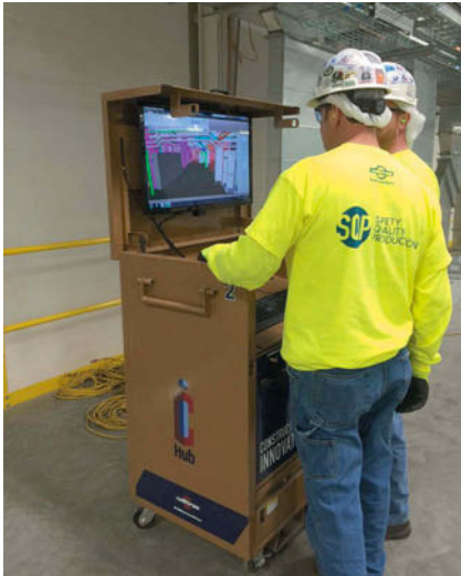
With the Ci Hub, anyone on the installation/construction team can pull up the most current 3D model and digital drawing sets when and where they need them.
